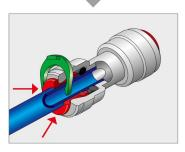
When no play is desired for the fitting and tube, use our company's LC to eliminate the play of the fitting.
