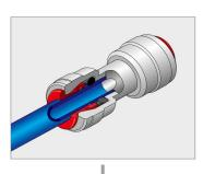
To make sure that the fitting is properly connected to the tube, pull it once.
