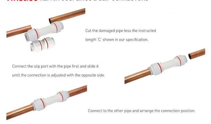
Twistloc repair couplings are designed to be suitable for use on copper, PEX and PB pipe offering the installer the ability to easily repair damaged pipework.
