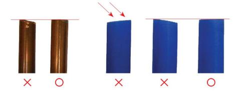
When cutting tube, ensure that the ends are cut squarely and free of burrs.
